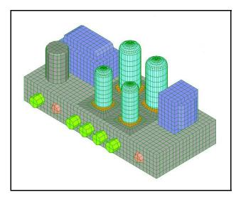
After applying heat generation, convection and radiation properties to the FEA model the simulation was performed, the results of which are described below.
