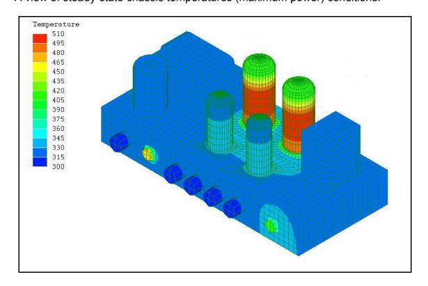
To reveal maximum temperatures within the assembly, we can employ a "cutting plane", virtually slicing through the amplifier and revealing the interior temperatures of the output vacuum tubes under full drive.
