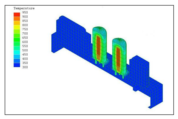
Temperature color codes, temperature scales and the "cutting plane" are userdefined in this particular FEA application. As expected, maximum temperatures are found within these two vacuum tubes.
